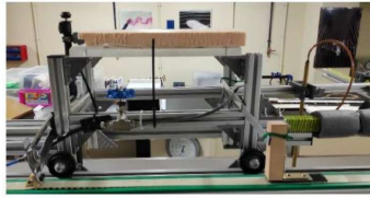
Figure 2.3: Cart on the top of the tunnel.
