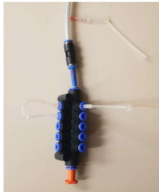
Figure 2.13: Flow distribution fittings and manifolds.
