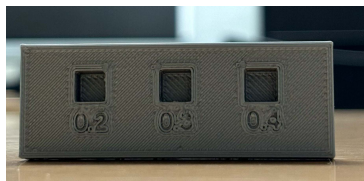
Figure 3.9: Square holes test.
