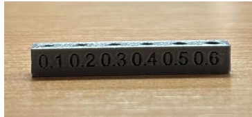
Figure 3.6: Tolerance holes test.
