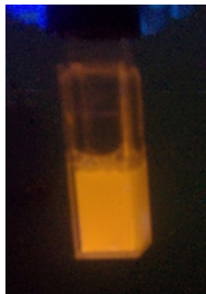
Figure 3.6: Photoluminescence of 1mg of micro-pSi functionalized with heptene suspended in 2ml toluene.
