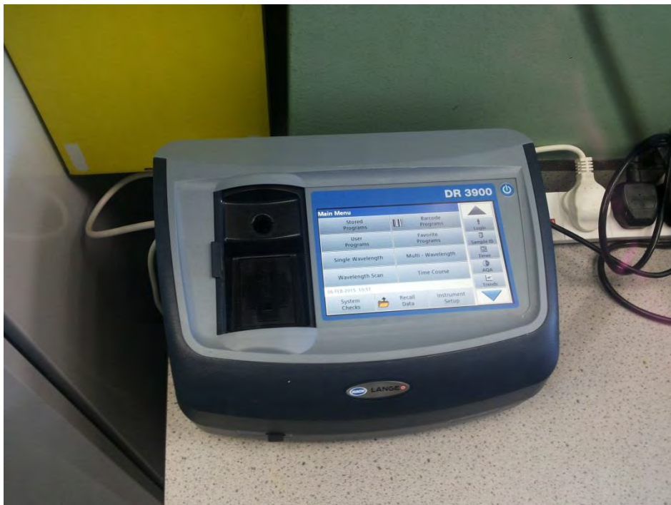
Figure 2.15 The machine used to read the results of the COD and VFA analysis.
