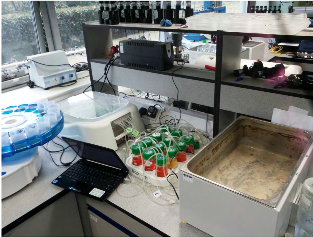
Figure 2.11 Set of equipments that composed the AMPTS.
