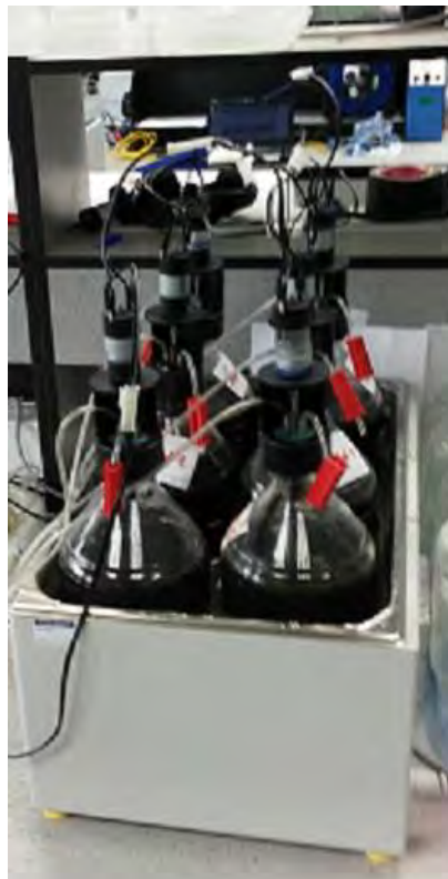
Figure 2.12 Water bath with the 2 liters bottles inside.
