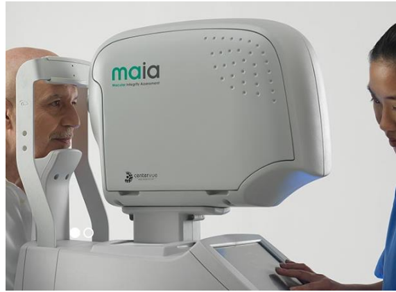
Figure 2.4: MAIA, an example of microperimetry device produced in CenterVue SPA, represents the latest advance in confocal microperimetry. Retinal images are acquired by Scanning Laser Ophthalmoscopy (SLO). An eye tracker allows accurate, real-time, compensation of eye movements. Luminance levels are compliant with existing standards (1000 asb.).
