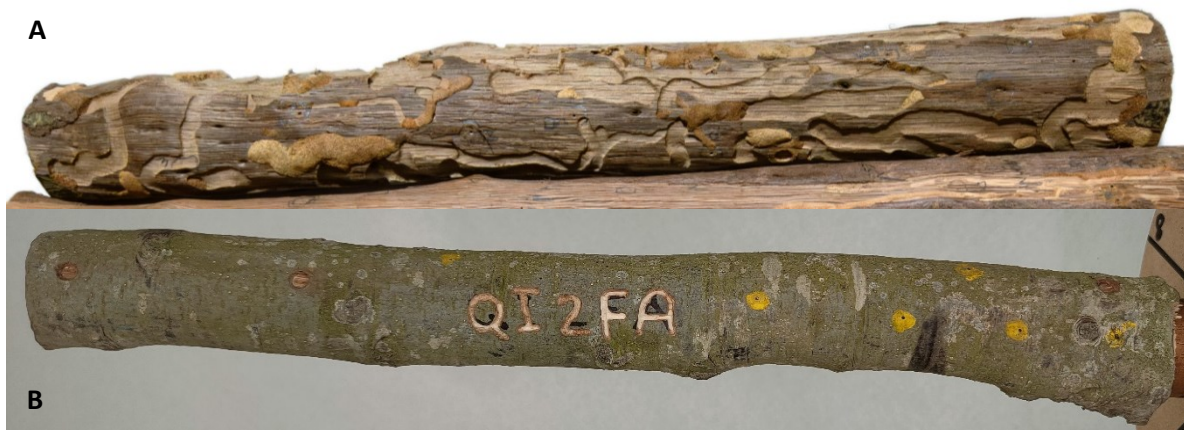
Figure 3.20. Log QI2FA, photo taken (A) after the heat treatment, losing all the bark, and (B) before the heat treatment, with the bark still on and all the holes colours visible.
