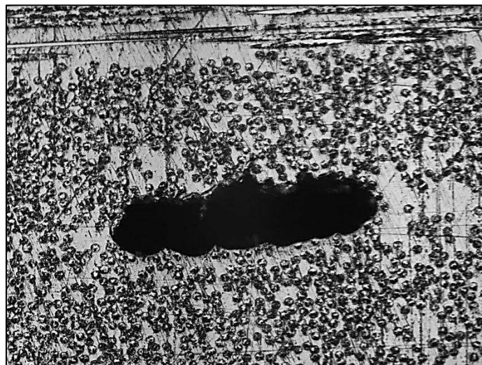
Figure 5-4. Enlargement of the porosity in the +60° layer
