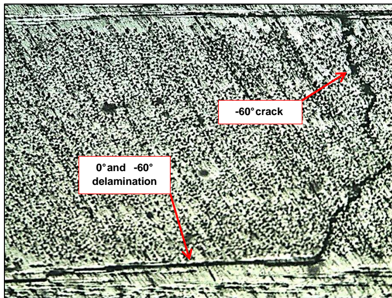
Figure 5-20. Enlargement on the -60° layer. The delamination between 0° and -60° layer is highlighted
