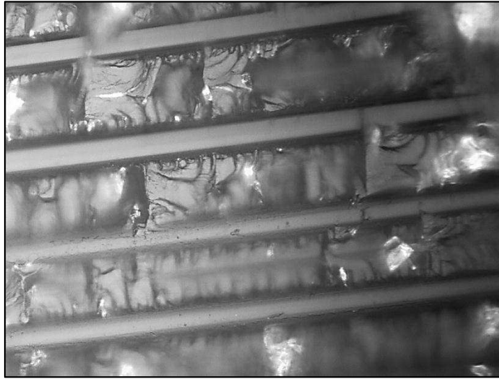
Figure 4-8. Optical microscope image of delamination surface of sample S-01. Zoom 50x
