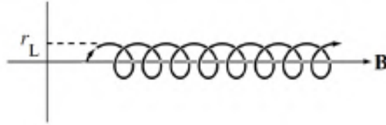
Figure 1.5: Particle confinement along the induction magnetic field line B .
