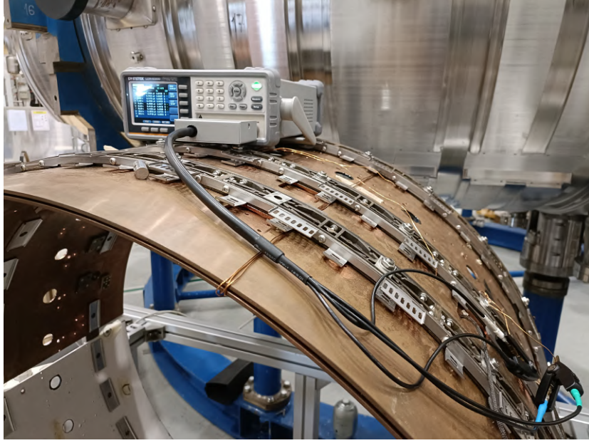
Figure 4.14: Coil inductance measurement setup.
