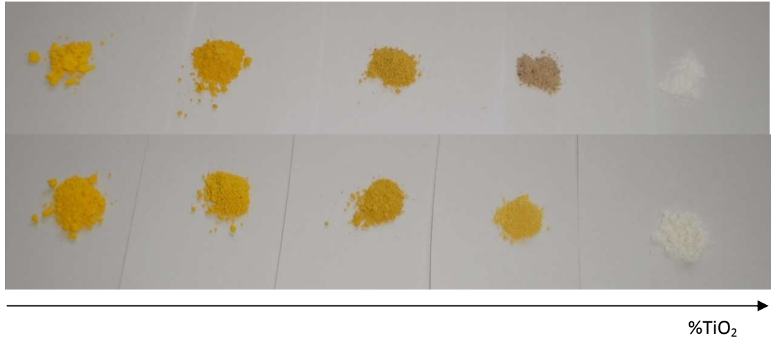
Fig. 22 Color change in the products. The upper row is formed by the hydrothermal compounds, the lower by the calcined compounds, with increasing amount of titania from the left to right.
