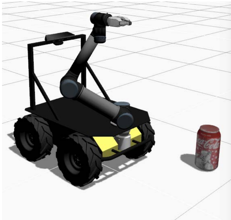
Figure 6.6.: The utilized robot. Husky UGV, UR5 robot arm, 2 Finger Gripper and Microsoft Kinect
