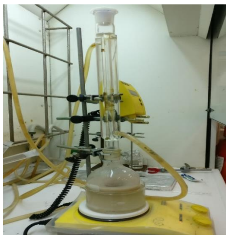
Figure 2.18. Reflux system to avoid the loss of ethanol during core-shell synthesis.
