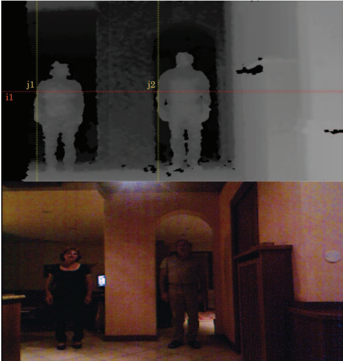
Figure 3.2. Example of detection of two people belonging to the same depth level. The dotted red line is the scanning of the algorithm at row i_1 whereas the dotted yellow ones represents the detection columns j_1 and j_2 .
