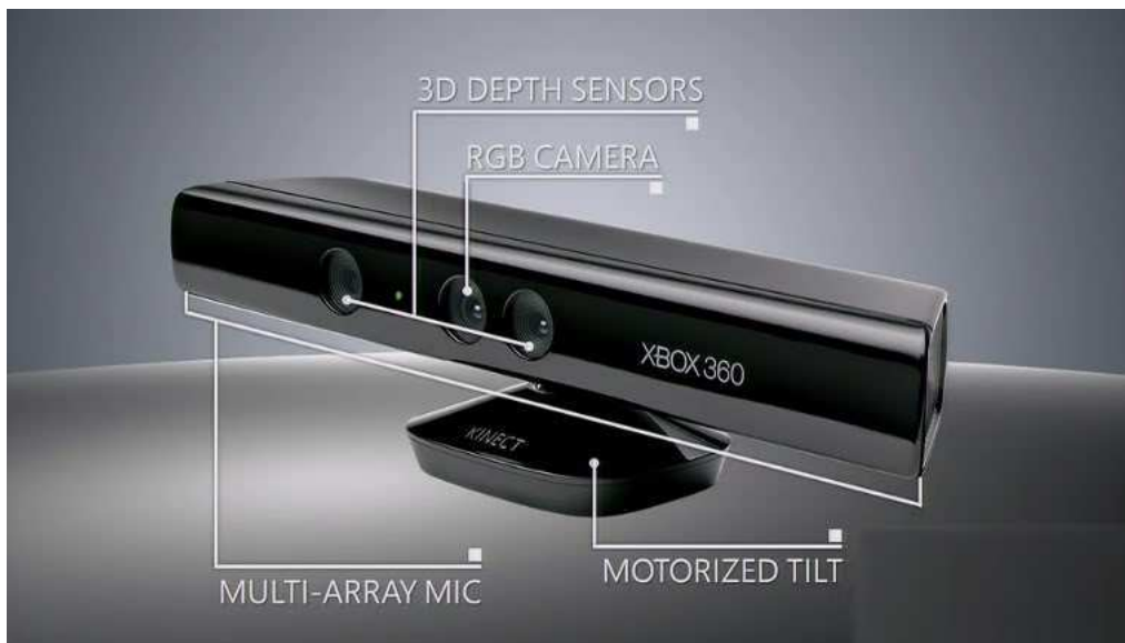
Figure 1.1. The Microsoft Kinect and its parts.
