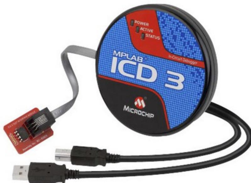
Figura A.7 Microchip MPLAB ICD 3
