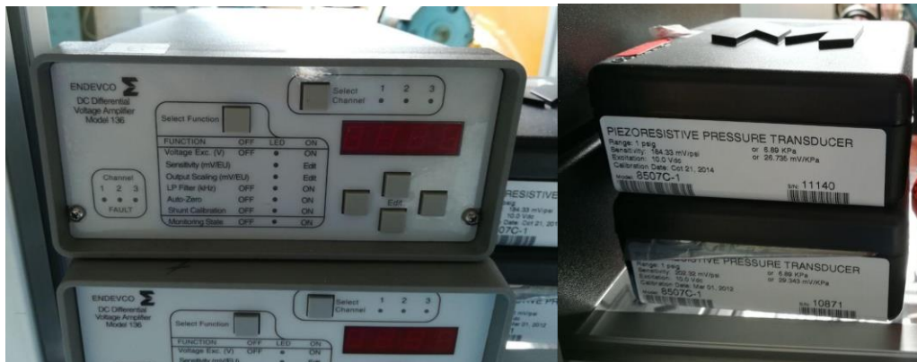
Figure 20: Signal amplifier and piezoresistive pressure transducer
