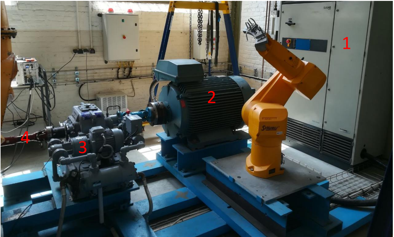
Figure 3: Electric box (1), electric motor (2), speed multiplier (3) and universal joint (4).
