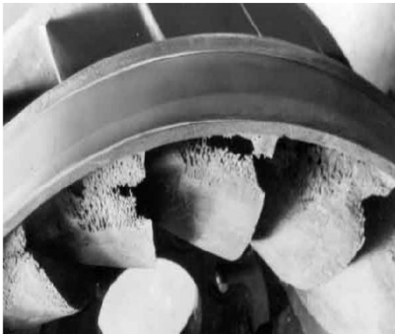
Figure 2-6: Typical damage of cavitation in a Francis turbine runner [10].
