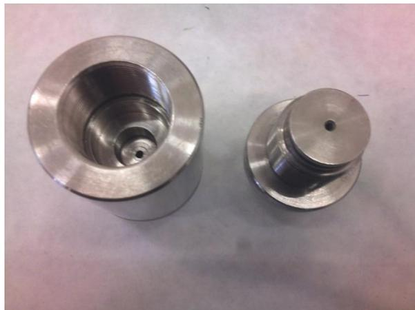
Figure 2.5: Extraction Cell
