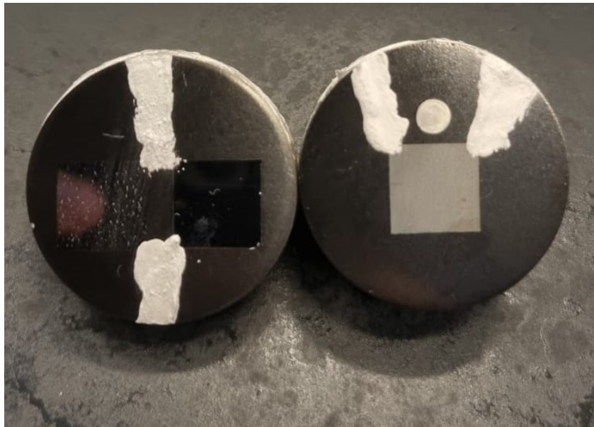
Figure 29: Samples after preparation with silver paint.
