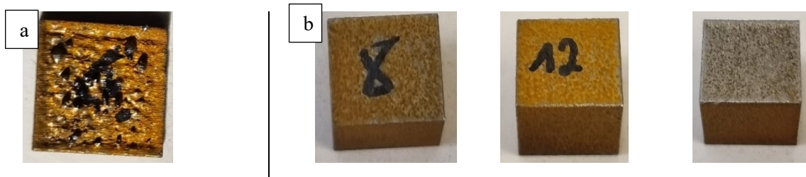
Figure 23: Samples used in this work. a) one of the six samples that could not be fully printed; b) the three selected samples used for further characterization.
