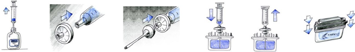
Figure 29: a schematic representation explaining how to fill a cartridge. (from left to right)
