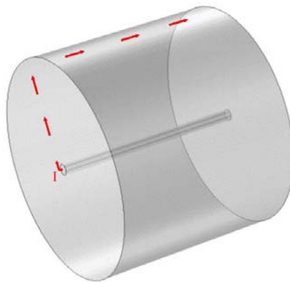
Fig. 5.2 Model of a conductor. Return of current through the external domain.
