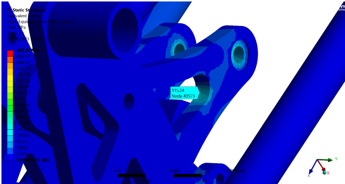
Figure 8.8 – Stress on Lift Up System
