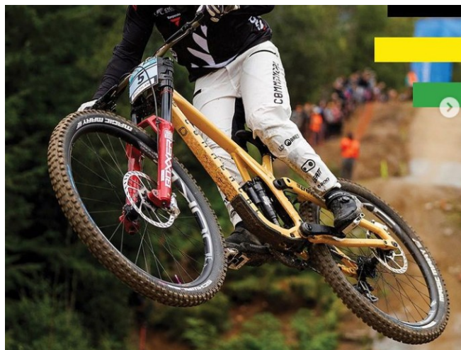
Figure 5.1 – MTB with air Monoshock
