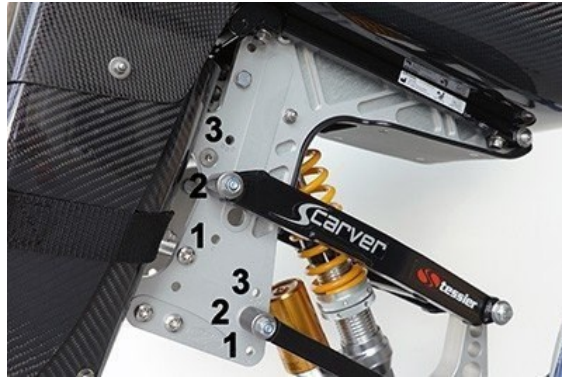
Figure 4.1 – Scarver's kinematic configurations
