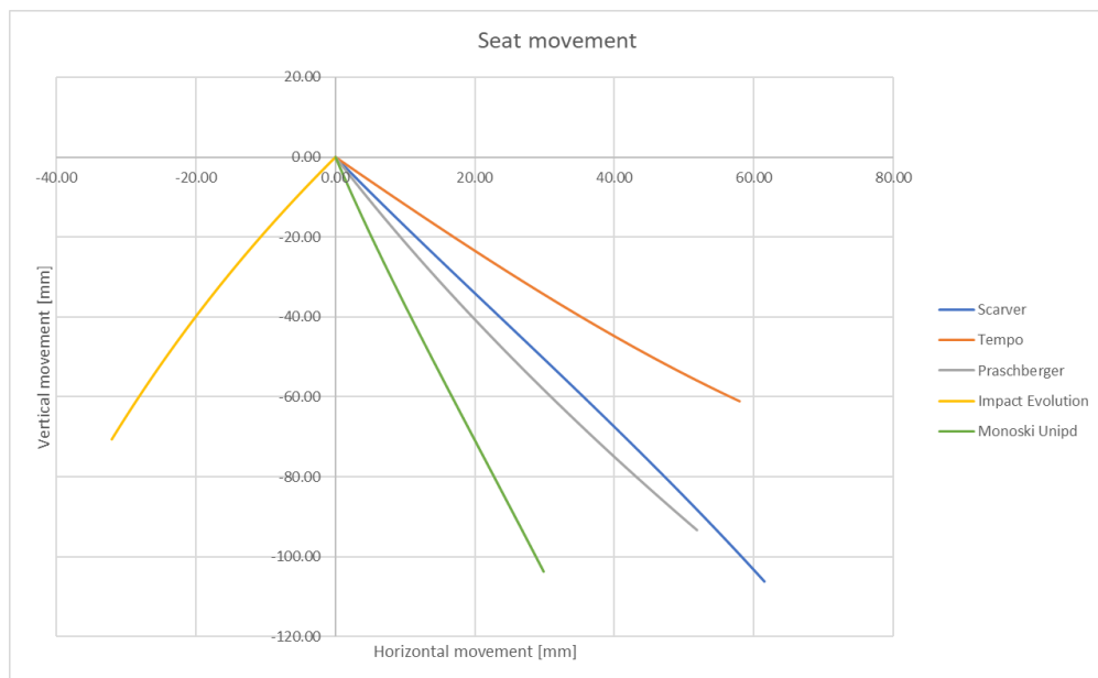
Figure 6.3 - Monoski Unipd seat movement comparison
