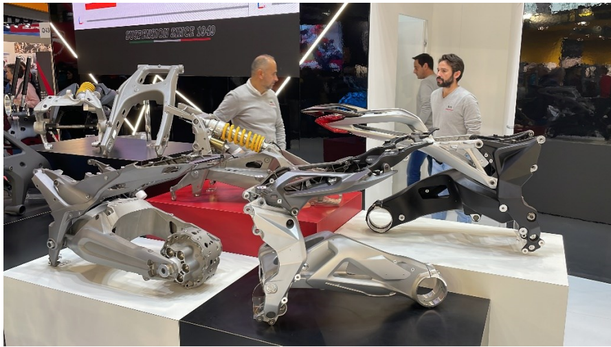
Figure 7.3 - Motorcycle components made by die casting
