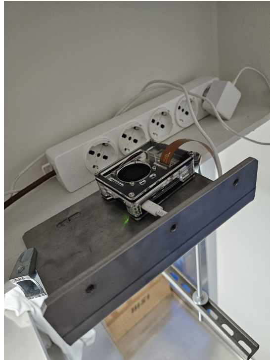
Figure 3.15: Raspberry Pi 5 installed on Site 2 inside a protective case with active cooling.
