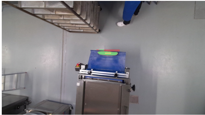
Figure 4.10: Example of bad clustering input. The color-based clustering stage includes an additional region in the upper-left area that is chromatically similar to the dough but does not belong to the actual product surface.
