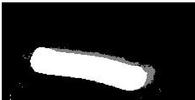
Figure 3.4: Example of the motion detection module at Site 1, showing a dough ball passing through the monitored area and activating the trigger used to store the corresponding RGB-D frame for dataset creation.
