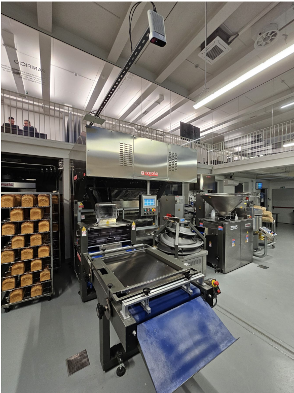
(a) Site 1: output area where dough balls are released and collected on the blue table
