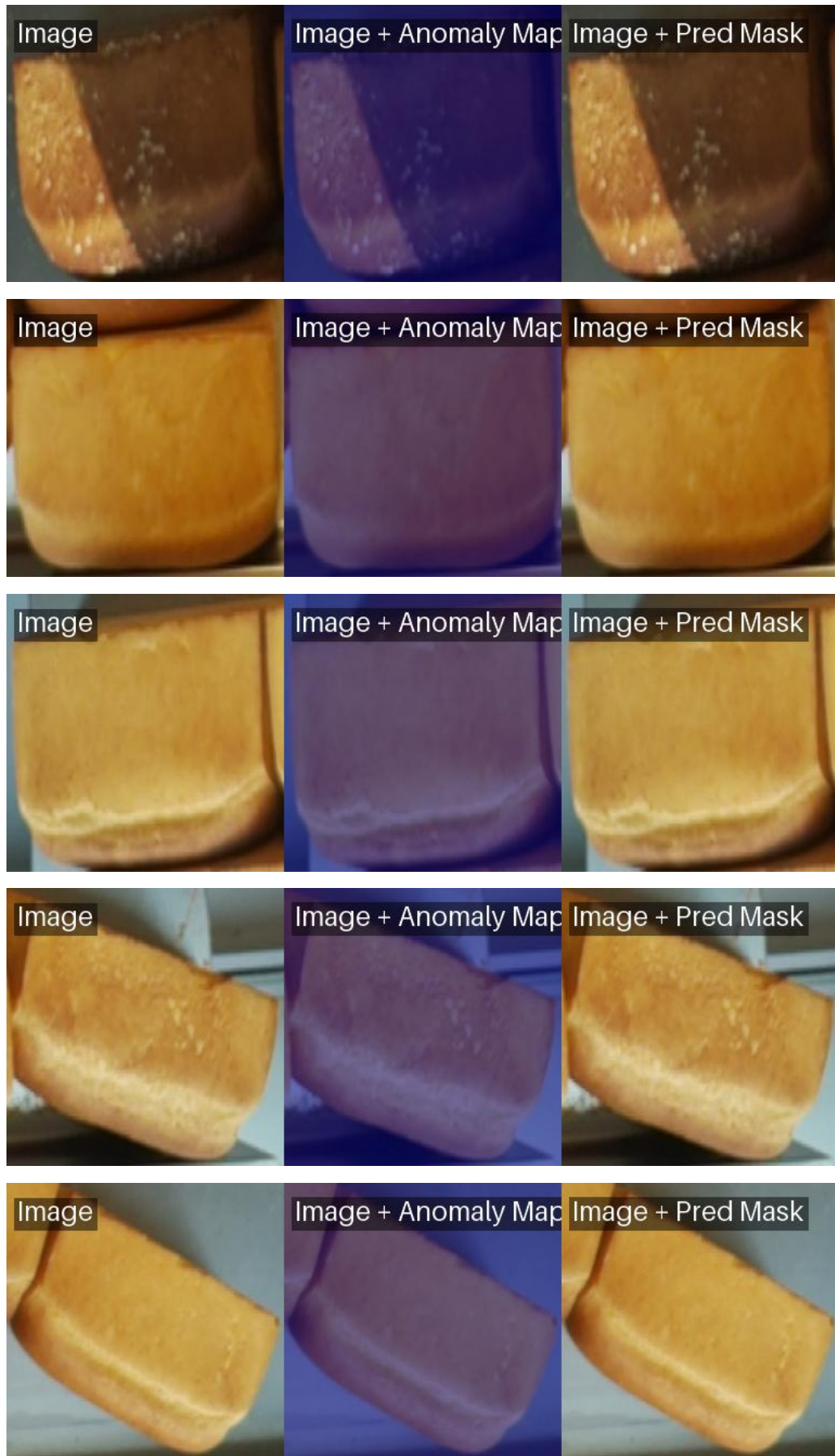
Figure 5.16: Compact qualitative visualizations exported by the inference pipeline for five representative good bread samples. In these cases, the heatmaps remain very flat and the predicted anomaly masks are negligible, consistently with the low anomaly scores observed in the quantitative analysis.
