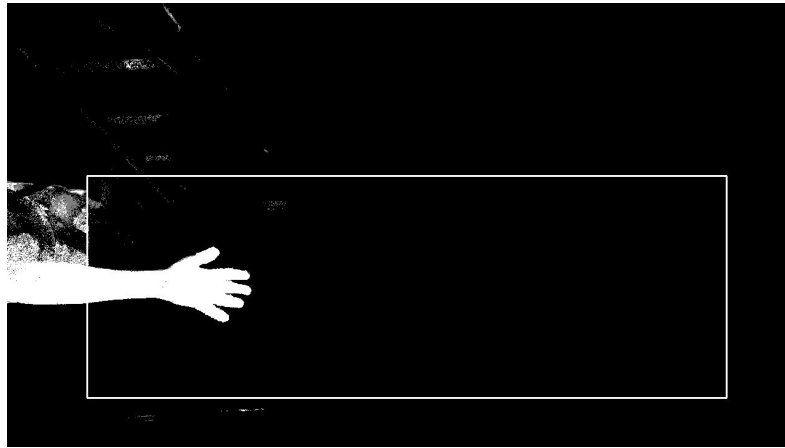
Figure 3.3: Example of a configurable region of interest (ROI) superimposed on a background-subtraction mask. Although this example refers to the Site 2 workstation shown in Figure 3.13, it illustrates the same motion-triggering principle adopted for data acquisition at both sites. The white region corresponds to the detected foreground, while the black region represents the background.
