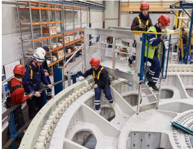
GE HALIADE – 6 MW 900 V (3x3 phases) – 256 poles (PMs) – 144 coils/phase Diameter 7.6 m – Weight 150 tons Water cooling
