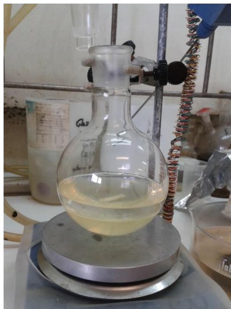
Figure 3.9 Washing of [bmim][Cl] with ethyl acetate. The system is biphasic, with the ethyl acetate on the top and the [bmim][Cl] on the bottom.
