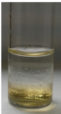
Figure 5. 1 Triphasic mixture (reaction 12): the upper layer is the ether phase, in the middle there is the water phase, while the lowest layer is the IL phase
