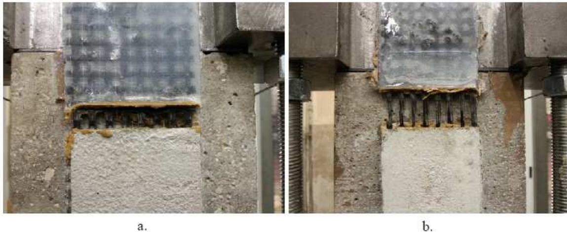
Figure 3. a) Slip of the fibers in specimen DS_CW_330_60_3. b) Stretching of the fibers at the cementitious matrix-epoxy interface in specimen DS_CW_330_60_1.
