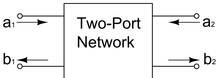
Figure 1.8: Two-port network model
