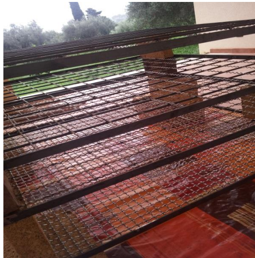
Figure 4.1. Screening utilized for the merceological analysis of the residual waste
