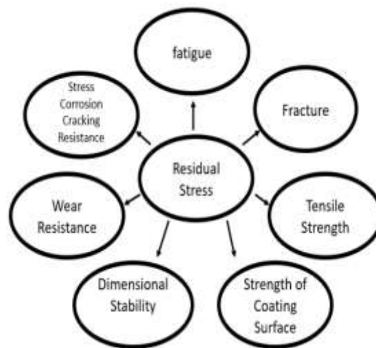
Figure 9: shows the parameters affected by residual stress [16].
