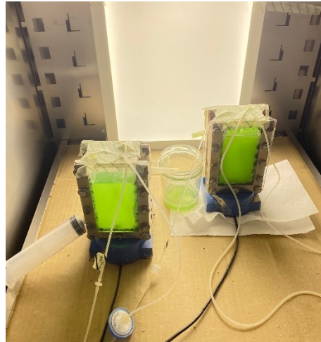
Figure 2.4. Experimental set-up for mixotrophic cultivation.
