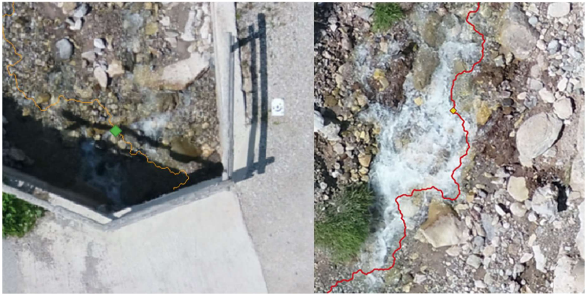
Figure 87: On the left the only Step-pool found at “Meto Valle” for \Delta x = 20\text{cm} , while on the right a riffle found for \Delta x = 40\text{cm}
