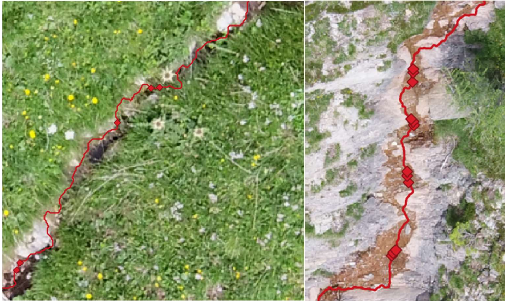
Figure 99: On left an example of extra point caused by grass and on right side the problem due to the waterfall at “Affluente 1”
