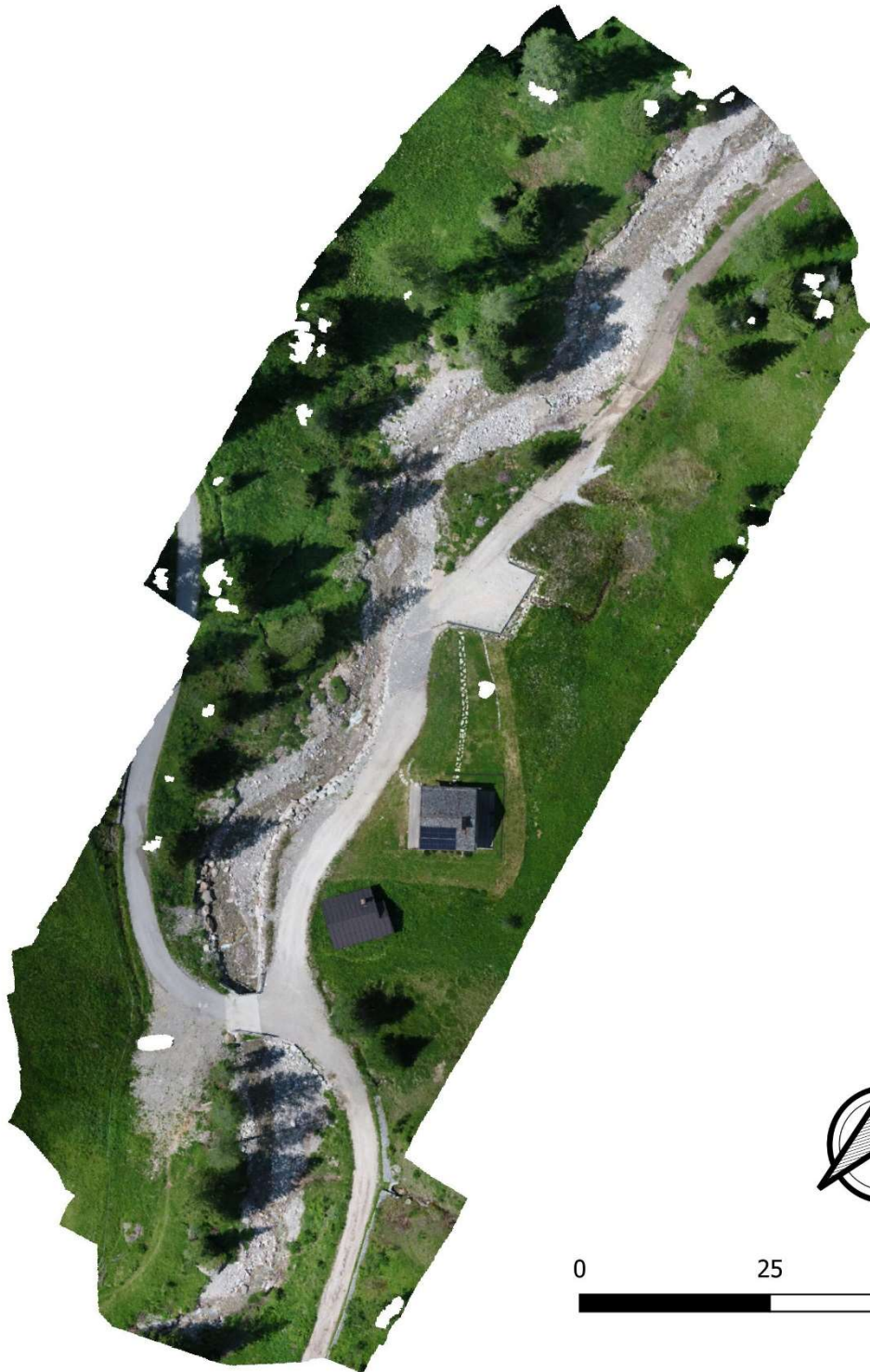
Figure 82: Orthomosaic of "Meteo Valle" with ground resolution di 7.21 mm/pixel
