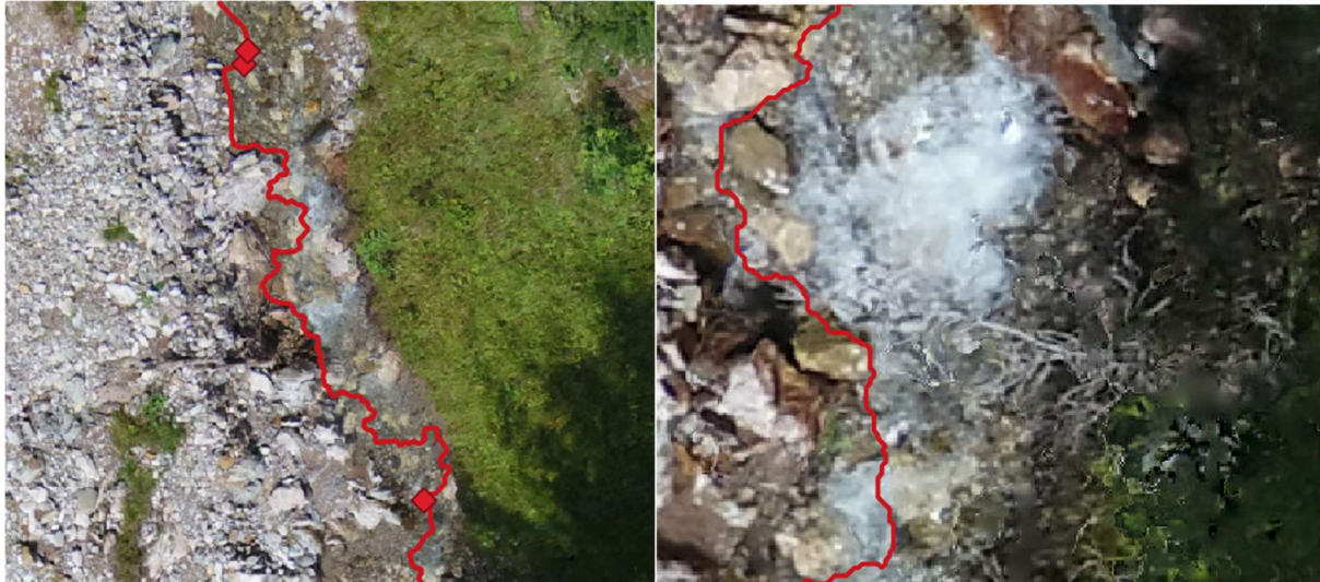
Figure 149: On the left side an example of extra points due to distortion of DEM on “Ponte Downstream”, while on the right part a missing point
