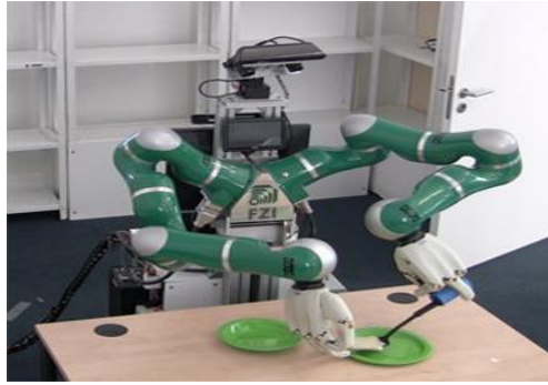
Figure 2.1 Two Kuka robots simulating human arms
