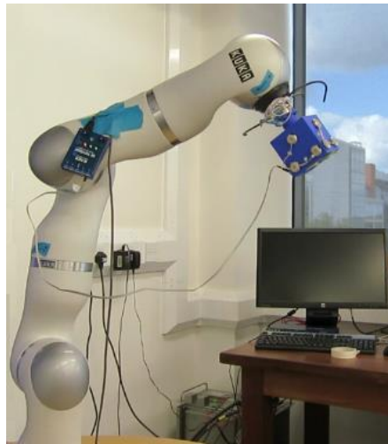
Fig.4.2: KUKA robot with the sensors mounted
