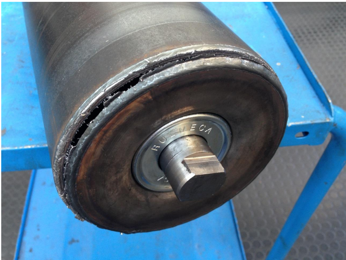
Fig.4.16 Typical failure of the rollers. The crack propagates from the crack tip due to the lack of penetration in the weld joint.
