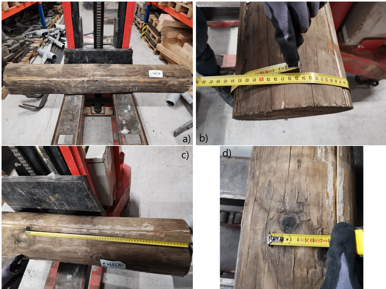
Figure 4.1.3: a)Preparation of the specimen; b)Identification of the sample head; c)Position of the knot; d)Knot size.
