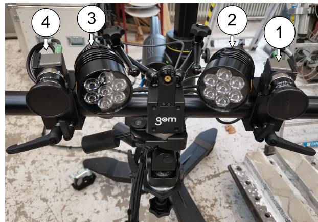
Figure 4.2.8: DIC camera set-up: 1) polarizing filter of the camera; 2) polarizing filter of the led-lamp; 3) polarizing filter of the led-lamp ; 4) polarizing filter of the camera.
