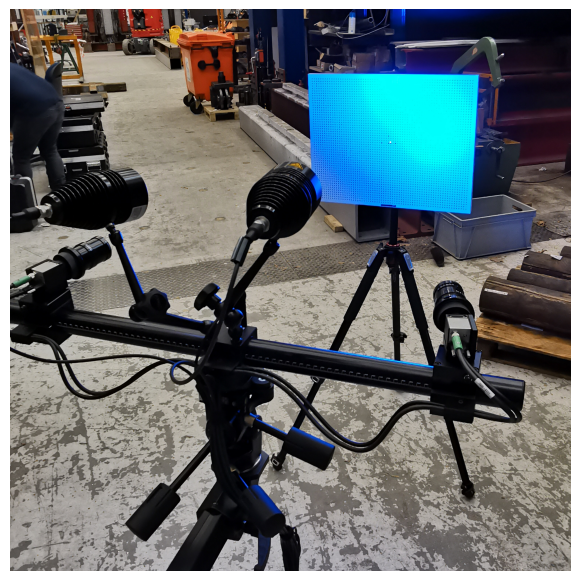
Figure 4.2.9: Calibration of the cameras.
