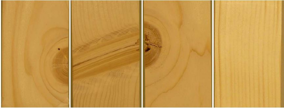
Figure 2.1.5: A knot seen from all four sides of a wood specimen 45 x 45 mm in square section [8].
