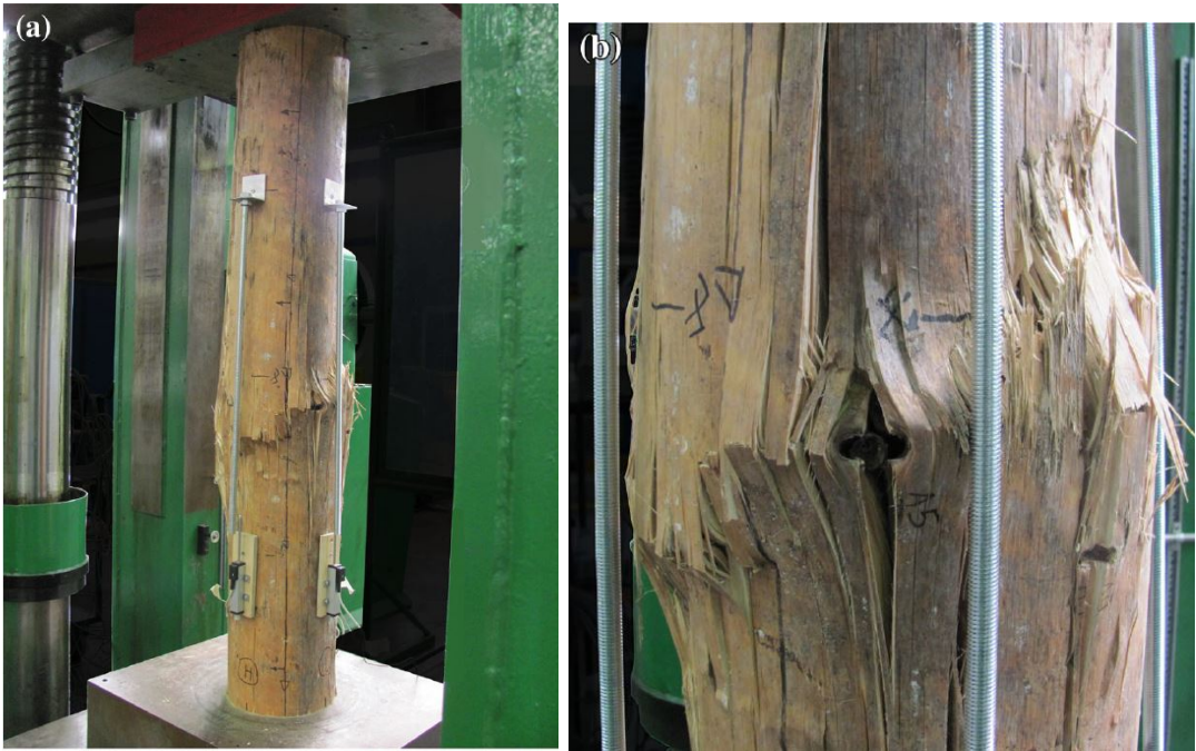
Figure 2.3.2: Failure appearances of dry pile specimens loaded in axial compression. (a) Total view of failed specimen. (b) Details of kink band and local buckling [2].
