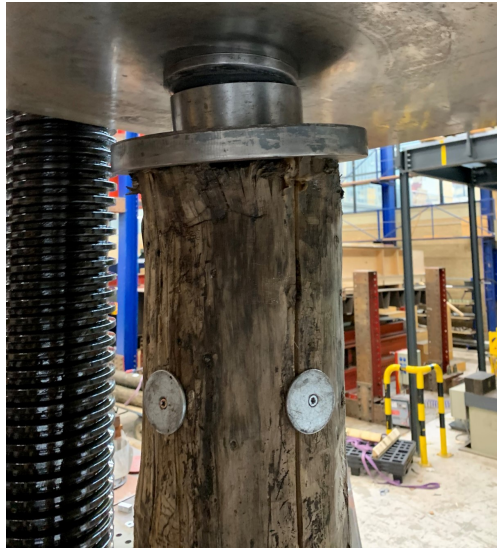
Figure 5.2.5: Failure by crushing of the surface of the test piece.
