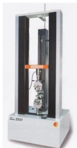
Figure 6.3 Galdabini SUN 2500 dynamometer
