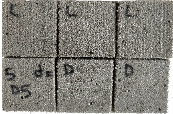
Figure 8.4 Biochar filled ample foams for the compression set. Samples in the first row have 5% wt. rice husks, while the second row's samples are filled with 5% wt. of Arundo donax
