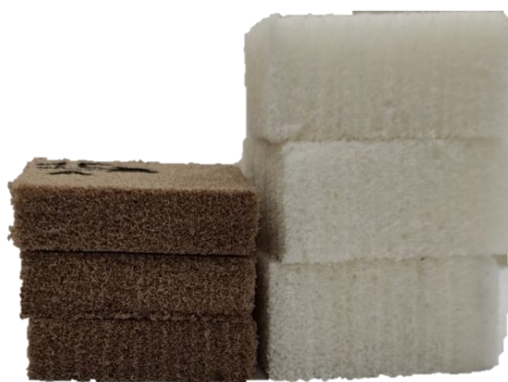
Figure 8.3 Compression set samples after running the test. Lignin based polyols foam on the left, reference on the right
