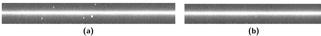
Figure 2.15: The same spectrum section before (a) and after (b) the cosmic ray removal.
