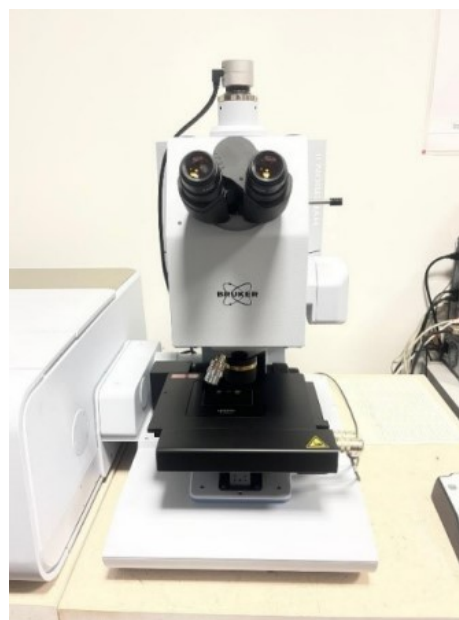
Fig. 6. Bruker Hyperion II FTIR microscope located at the University of Padova, Department of Geosciences
