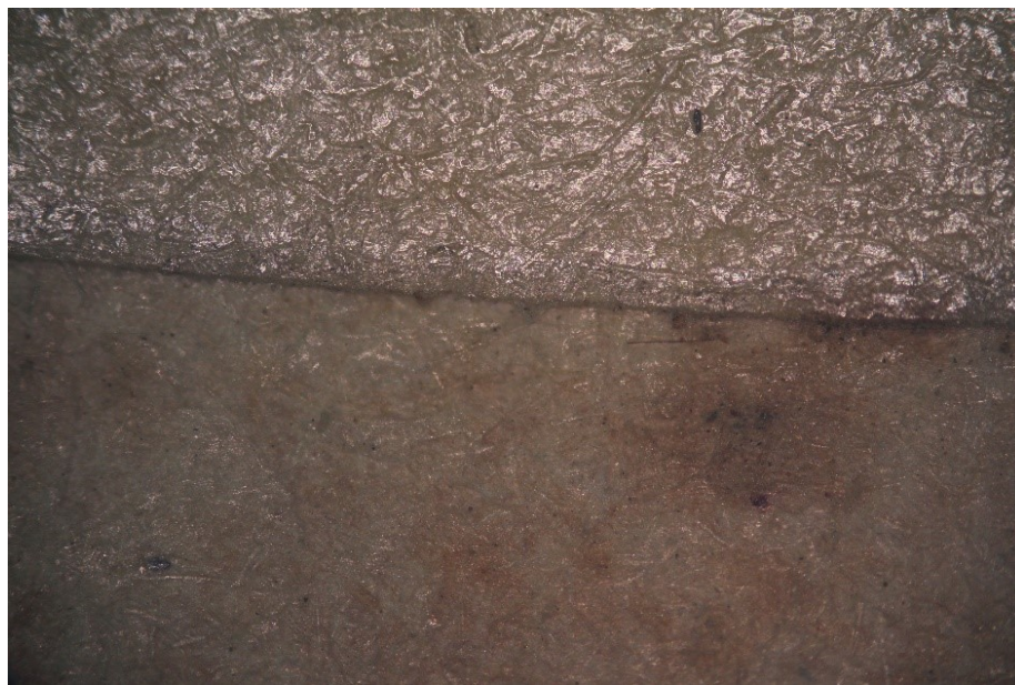
Fig. 12. The comparison between the surface of photo card and brown support shows the glossy surface of photo card. Optical Microscopy in 5x.
