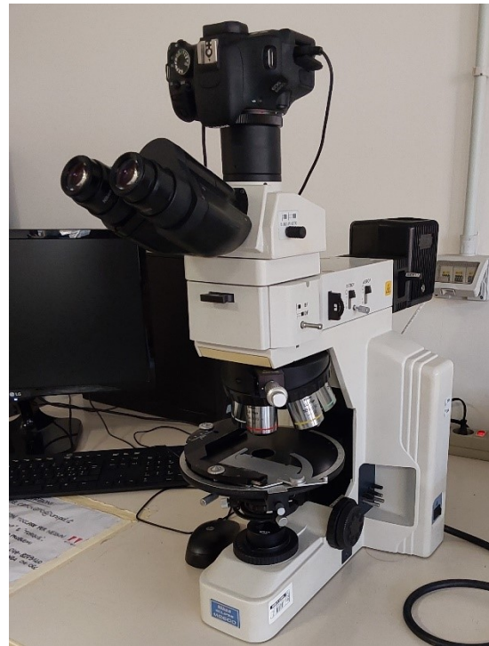
Fig. 3. The polarized microscope Nikon Eclipse ME600 with five objectives (5x, 10x, 20x, 50x and 100x) equipped with a Canon EOS 600D camera in the Geoscience department of University of Padova.
