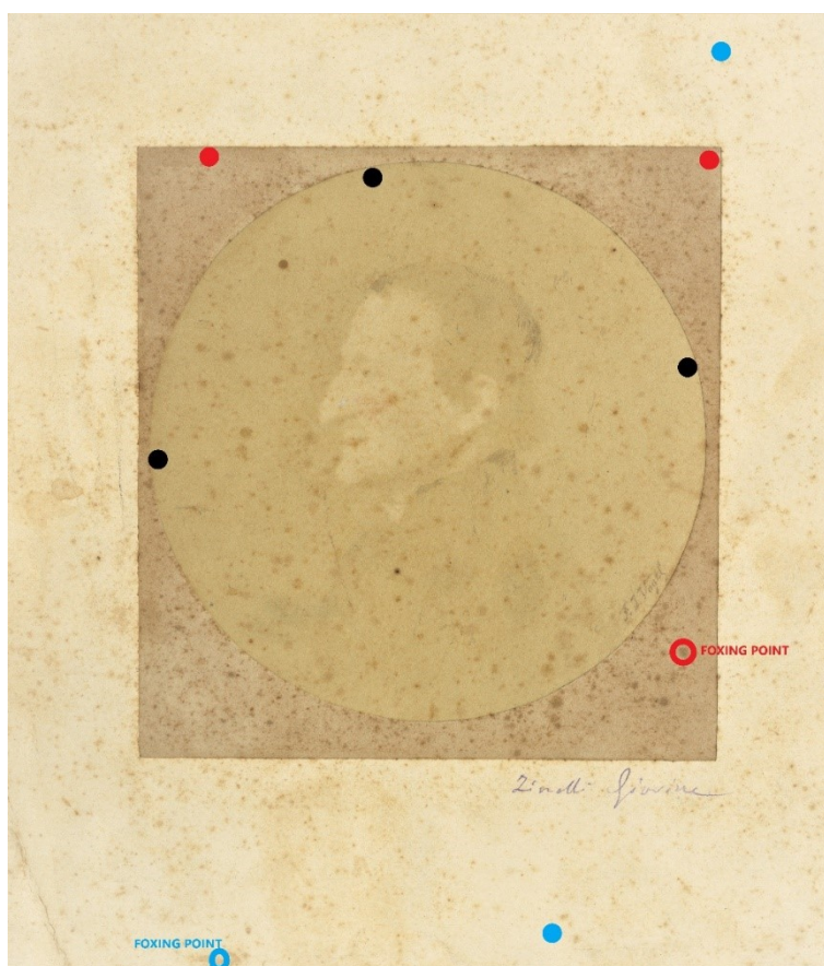
Fig. 18. Nine points chosen on the photo sample for the ATR-FTIR measurements. Black point from photo card. Red points over brown support and blue points on white support. Points with foxing alteration are marked.
