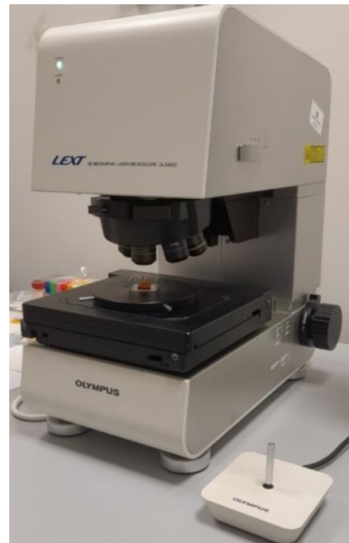
Fig. 4. Olympus LEXT OLS 4000 3D confocal laser scanning microscope in the Geoscience department of Padua University, courtesy of the CIRCe Centre.
