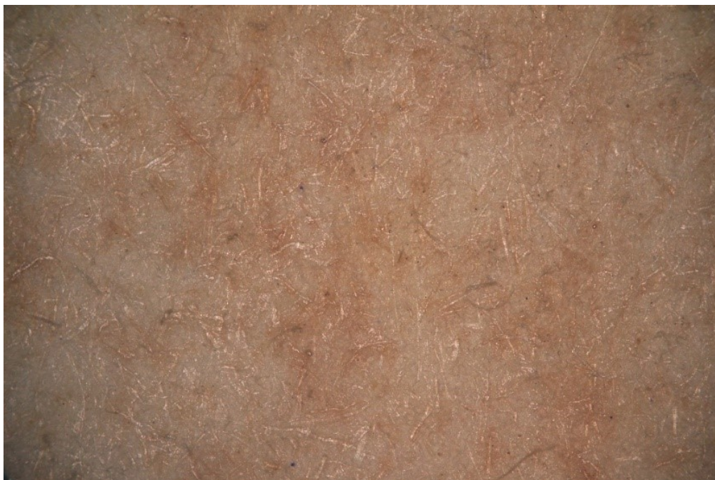
Fig. 10. Optical microscopy on the support layer, snowflake foxing; lighter with irregular shape. in 20x magnification
