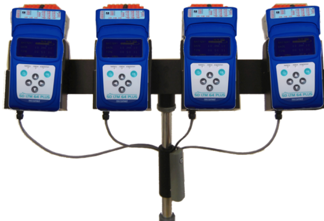
Figure 31: Example of synchronization of four headboxes to obtain up to 256 active channels for EEG acquisition
