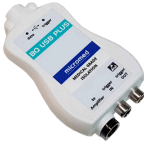
Figure 32: Example of BQ USB PLUS interface to connect headbox to PC for EEG trace acquisition
