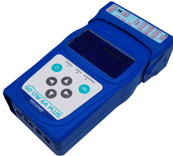
Figure 30: Example of SD LTM 64 PLUS Headbox: portable device for acquisition of electroencephalographic signal
