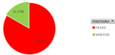
Figure 41: Test 2 failed as a result of millisecond rounding in Matlab. During this test it became clear that the problem was the rounding of milliseconds in Matlab
