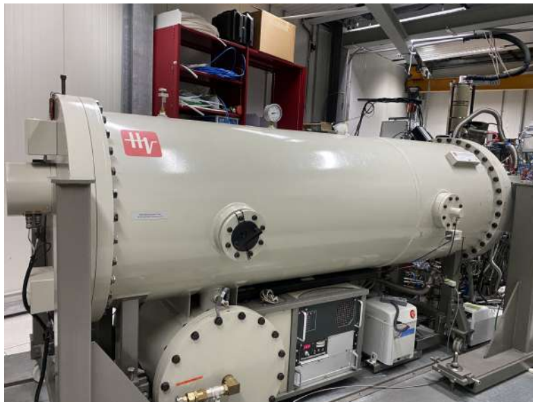
Figure 23: Accelerator installed at LUNA 400.
