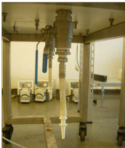
Figure 7.12 – Leachate extraction port
