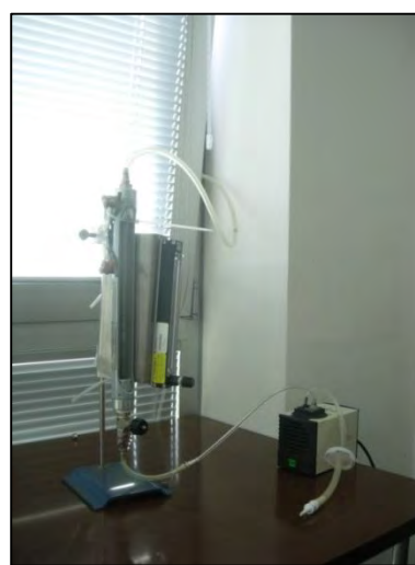
Figure 7.15 – Instruments for emptying the biogas sampling bags
