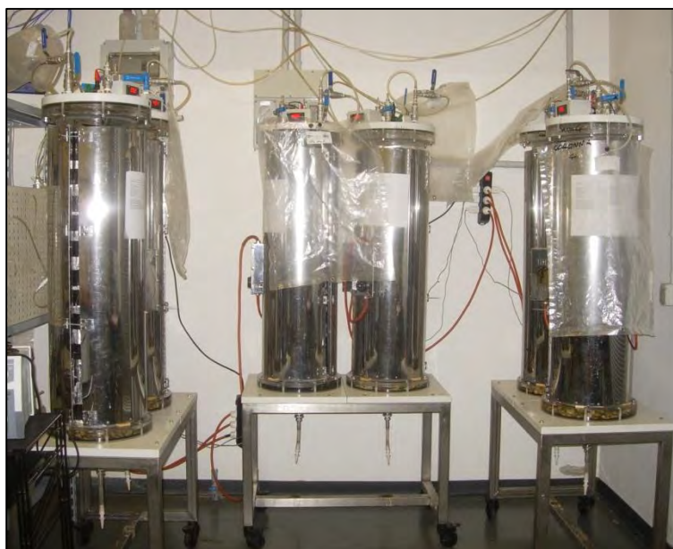
Figure 7.18 – Columns with thermal covers
