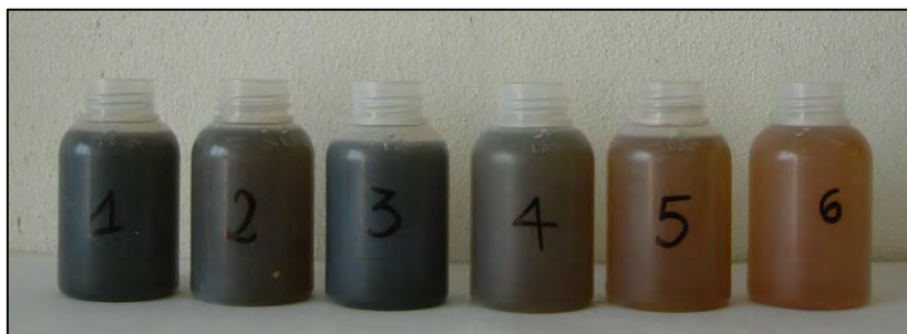
Figure 7.16 – Samples of leachate taken from columns for chemical analysis (08/10/14)
