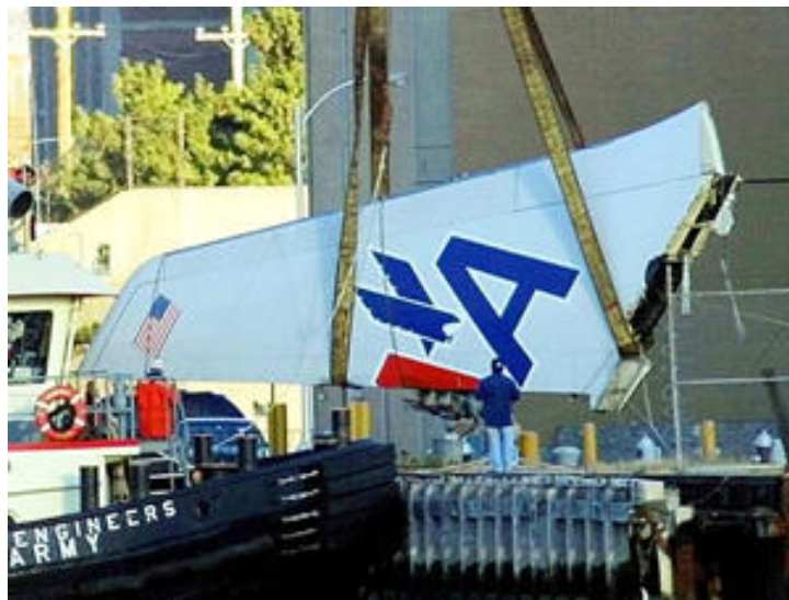
Figure 1.1: On November 12 th 2001, the American Airlines Flight 587 crashed shortly after takeoff because of a tail structure failure while encountering wake turbulence.
