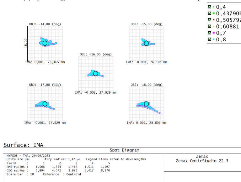
(b) Spot Diagram for the second Channel, Zernike terms up to Z_{16} .
