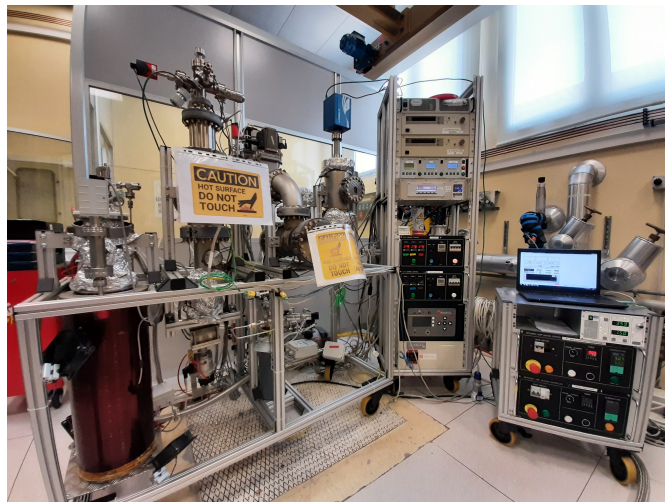
Figure 5.5: The three coating systems at LNL and their controllers. They are dedicated to (from left to right): 6GHz accelerating cavities (not used in this work), Nb_3Sn and NbTi . In the far right side there is the induction heating chamber equipped with a RGA.
