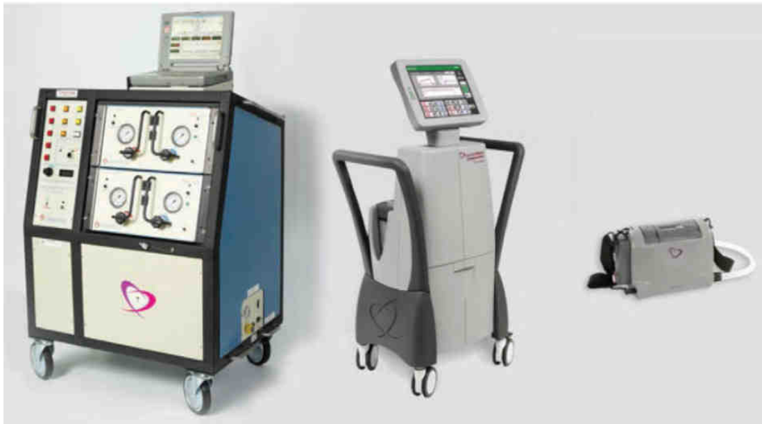
Figura 5.4 Drive unit a confronto :“BigBlue”, Companion e Freedom
