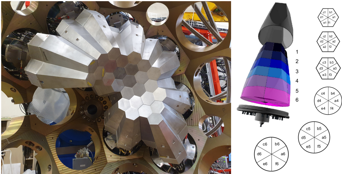
Figure 2.8: The AGATA array during its first commissioning at Legnaro National Laboratories in April 2022 (left). Schematic view of a single segmented HPGe crystal of the AGATA array (right). Right panel is taken from reference [4].
