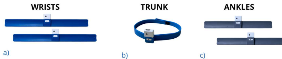
Figure 3.1: ARC Wireless Sensor Setup. a) Wrist supports with inertial sensors. b) Collar with inertial sensor. c) Ankle supports with inertial sensors.
