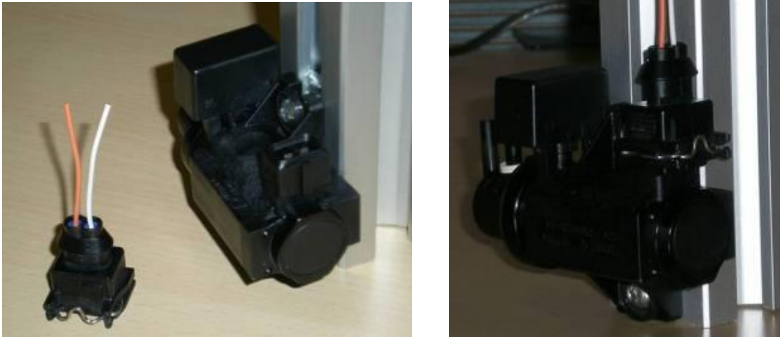
Figure 11: Plug and part separated (left) and correctly mounted (right).
