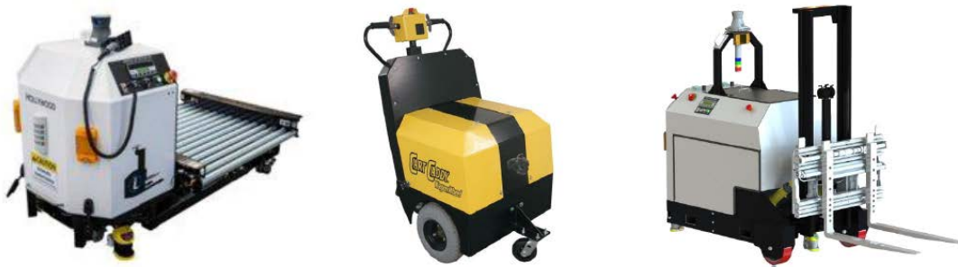
Figure 2.2: AGV examples: from the left, a unit loader, a tugger and a fork lift.
