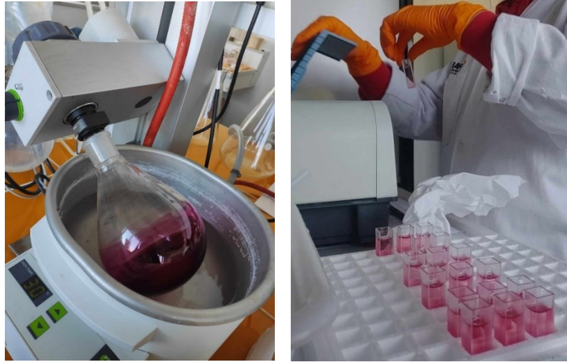
Figure 3.2 7: Extraction with the Buchi Rotavapor and measurement of the absorbance of total tannins
