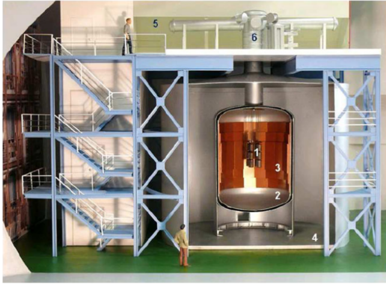
Figure 2.1: Artistic representation of the GERDA experiment (detectors not to scale): the germanium detector array (1), the LAr cryostat (2) with its internal copper shield (3), the water tank and the Cherenkov muon veto (4), the GERDA clean room (5) and the lock system (6) [12].
