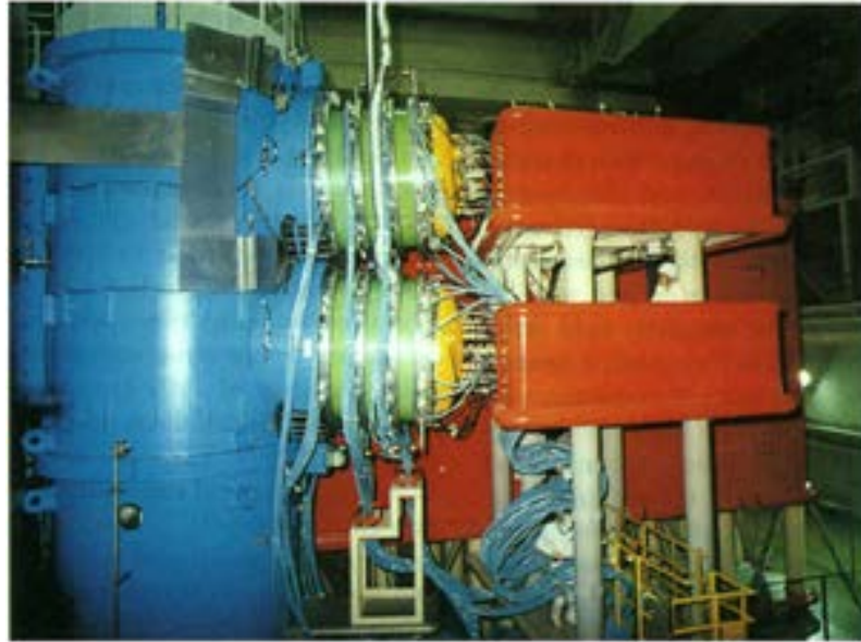
Figure 3.3: Detail of the JT-60 NBI system, showing the beam sources and the FRP rings [15].
