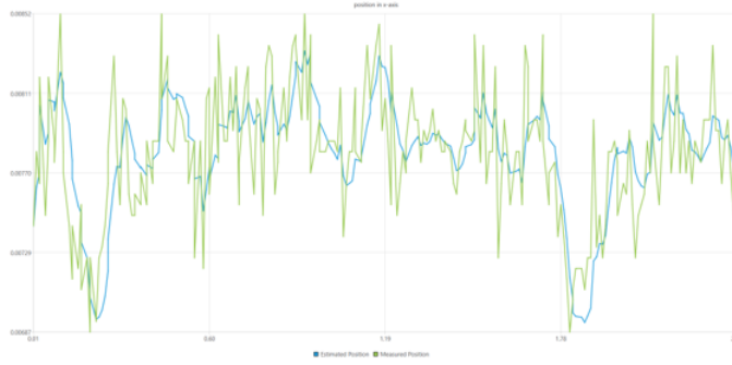
Figure 6.1: Trajectory of measured (green) and estimated (blue) position of the ball in the x -axis
