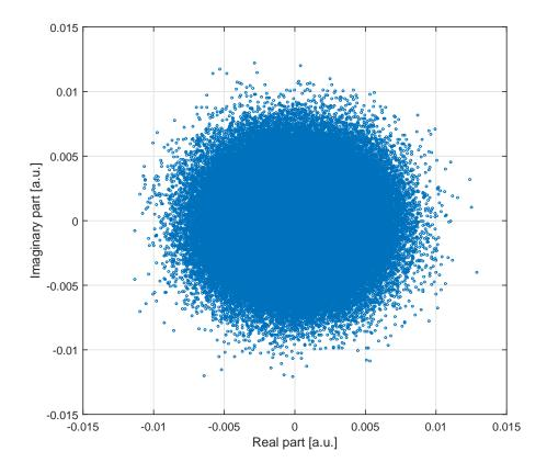
FIGURE 2.6: Graphical representation of one of the polarization components of the received signal after the optical front-end, the deskew operation and the orthonormalization. No equalization has been performed yet.
