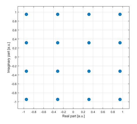
FIGURE 2.5: Graphical representation of the transmitted symbols for one polarization component.
