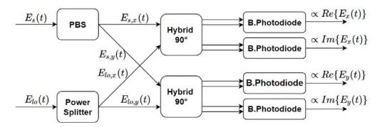
FIGURE 2.3: Schematic of a phase and polarization diverse receiver.  $E_{s,x}$ ,  $E_{s,y}$  and  $E_{lo}$  are the electric fields associated to the two polarizations x and y and to the local oscillator respectively.
