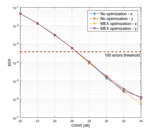
FIGURE 4.8: Performances of the CPR module before and after MEX optimization.
