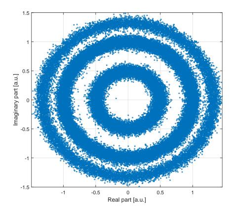
FIGURE 2.10: Graphical representation of one of the polarization components of the received signal after equalization.
