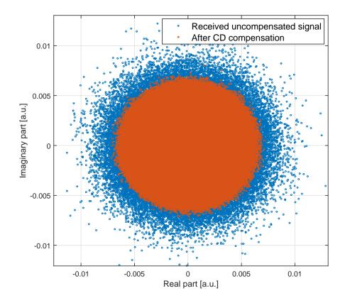
FIGURE 2.7: Graphical representation of one of the polarization components of the received signal after CD compensation.
