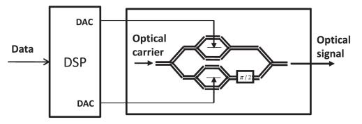
FIGURE 2.1: General scheme of a coherent transmitter.
