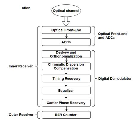
FIGURE 2.4: Complete logical scheme of a coherent receiver with all digital demodulator's modules listed
