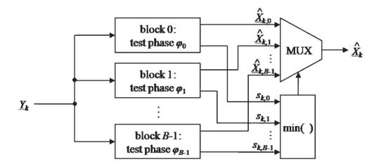
FIGURE 4.5: Feedforward carrier recovery using B test phase values  $\varphi_b$
