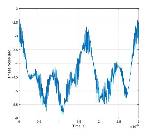
FIGURE 4.3: Example of the phase noise for a DFB laser with linewidth of approximatively 1 MHz  $\,$
