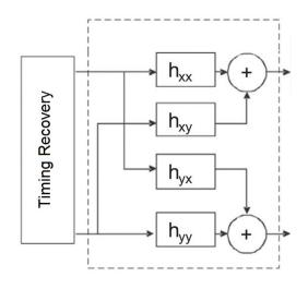
FIGURE 2.9: Butterfly structured equalizer with 4 FIR filters used to compensate polarization impairments.
