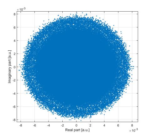
FIGURE 2.8: Graphical representation of one of the polarization components of the received signal after timing recovery.
