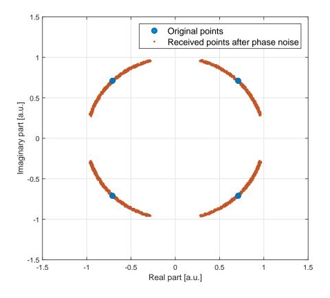
FIGURE 4.4: Effects of phase noise on the received signal
