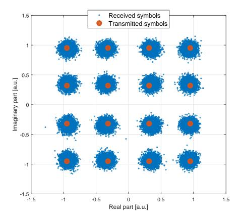
FIGURE 2.11: Graphical representation of one of the polarization components of the received signal after carrier phase recovery.
