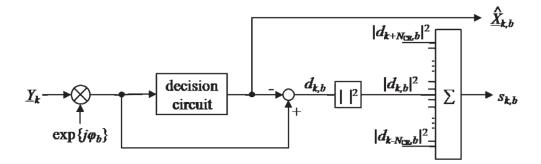
FIGURE 4.6: Insight of the test phase block for the feedforward carrier recovery diagram
