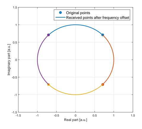
FIGURE 4.2: Effects of linear frequency offset on the received signal
